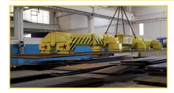
Lifting beams (with or without telescopic arms) able to handle sheets of different sizes, and of small (2mm) or greater thicknesses.
