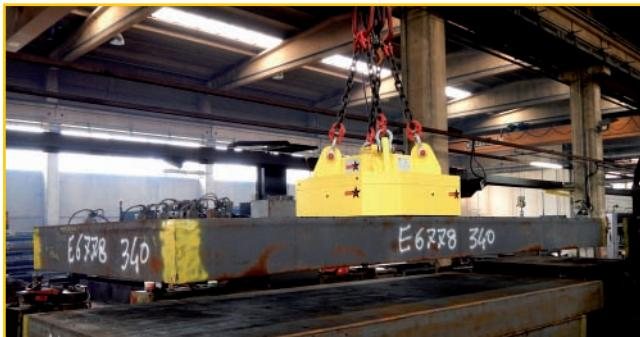
The well-structured SEP lifters, specially designed for the handling of slabs and forged blocks with an increased air-gap, are able to withstand high stresses and strains and are therefore extremely reliable over time.
