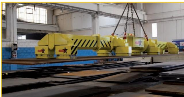
Lifting beams (with or without telescopic arms) able to handle sheets of different sizes, and of small (2mm) or greater thicknesses.
