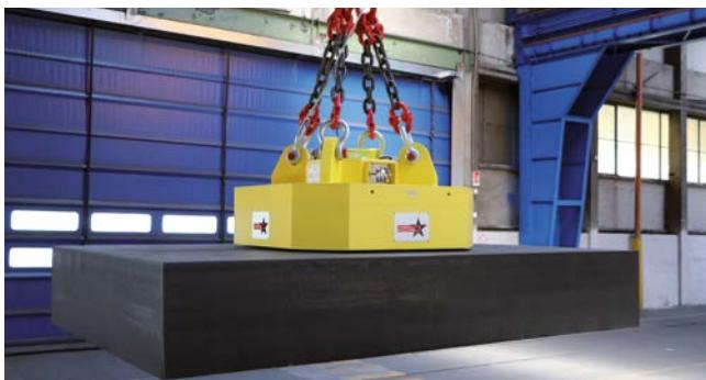
**Electro permanent lifters for the handling of slabs and forged blocks with an increased air-gap.**
