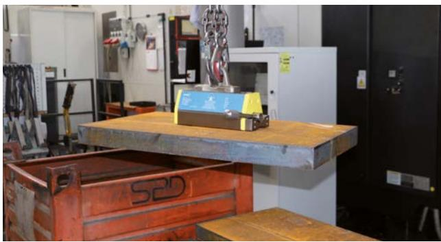
**Magnetic neodymium lever lifters suitable for handling both flat and round ferrous loads.**
