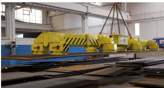
**Electro-permanent, fixed and telescopic beams, designed for handling sheet metals of all sizes, both small and large thickness.**
