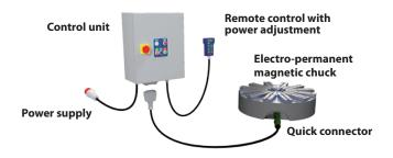
The electro-permanent chucks for turning operations are supplied with an electronic control unit featuring a remote power control panel with power adjustment, and with sturdy quick connector and watertight closure for the work machining phases. The holes for fastening the chuck to the machine are included.
