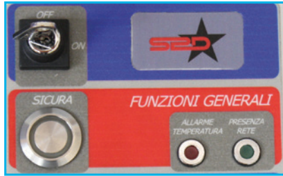
Safety button Temperature alarm Voltage presence indicator
