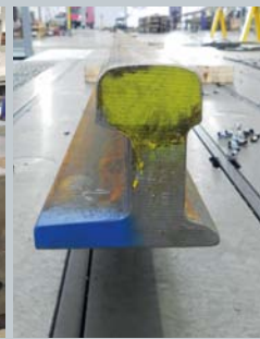
The high safety of the workholding magnetic system is guaranteed by electropermanent technology by SPD. Right side: geometry of the rail to be machined.
