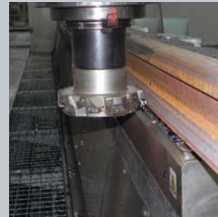
Machining operation of the foot. Right side: second processing of the rail head. Processing that requires a safe clamping condition.
