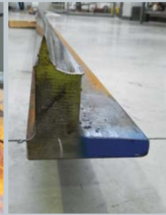
The high safety of the workholding magnetic system is guaranteed by electropermanent technology by SPD. Right side: geometry of the rail to be machined.
