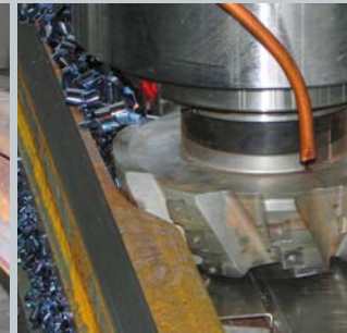
Machining operation of the foot. Right side: second processing of the rail head. Processing that requires a safe clamping condition.
