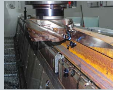
First operation of the rail head. Right side: profile of the rail being machined in one set-up only.
