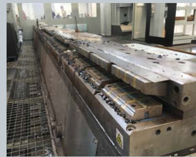
The high safety of the workholding magnetic system is guaranteed by electropermanent technology by SPD. Right side: geometry of the rail to be machined.
